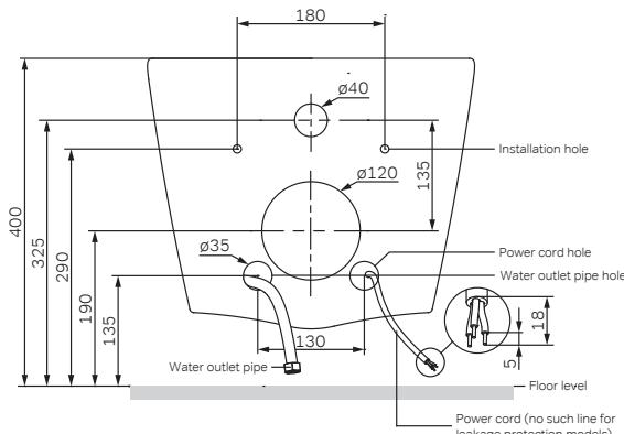
Put the toilet mat on the reserved position on the wall, direct the mounting hole of toilet mat to the fixed screw of the water tank frame, and then insert the mat, aligning with the flushing hole and sewage hole of the water tank, and pass the water outlet pipe through the water outlet hole, and the power cord passes through the power cord hole, exposed outside the wall.
