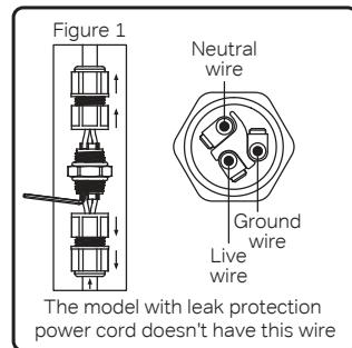
Install the power connector cable (no need to install the connector cable for the model with leakage protection plug), ambient light cable, knob cable, and microwave induction cable as shown in the figure. Note: When wiring, you need to disassemble the upper part of the waterproof plug, check whether the ground wire, neutral wire and live wire at both ends correspond to each other, and connect the power wire correctly.
