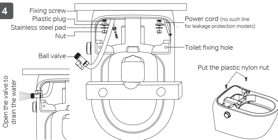
After the toilet is close to the wall, use a gradienter to measure the product to keep the product in a horizontal position. Then put a plastic plug and a stainless steel gasket on the fixed screw in turn, and then tighten the nut. Then connect the ball valve to the head of the outlet pipe and pass water to clear waste. Then put plastic nylon nut in the toilet fixing hole.
