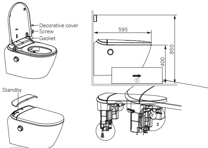
Fix the electronic seat on the top of ceramic, tighten it with the fixing screw, and install the decorative cover. after installation, take out the package in the direction of the arrow **1** in the figure. The remote control is installed at a distance of about 850mm from the ground, which is easy for users to remove it. When not in the use for a long time, press in the direction of arrow **2** to drain the residual water in the pipe.
