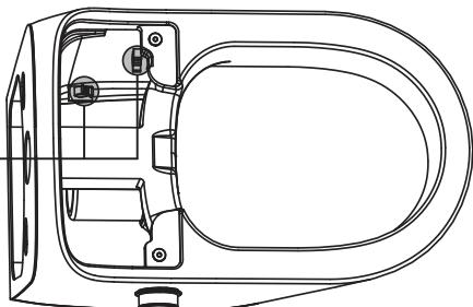
After the ambient light wire, knob wire and microwave induction wire are connected, arrange the wires and put them into the wire clip, and then press and hold the wire clip in the direction of closing indicated by the arrow. When you need to take out the wire, press the wire clip in the direction of opening indicated by the arrow.
