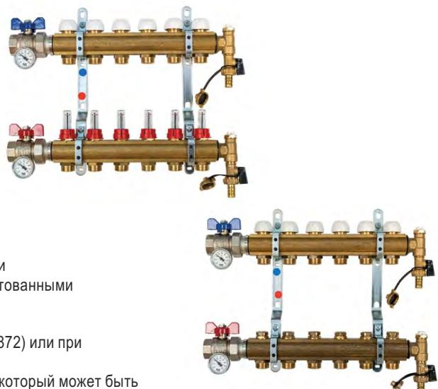
The Tiemme distribution units Art. 387... are a perfect solution for the heating and/or cooling systems installation. The distribution unit is available with 1" or 1"1/4 manifolds with 2÷12 ways 3/4"x18 Euroconus connection. The units are supplied complete of ball valves with holder for thermometer, air purge valves and drain valves.
