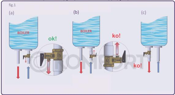
Before turning on the water heater, activate the control lever in the direction indicated by the arrow represented in fig. 1 so that the water begins to flow out of the drain. Then reposition the lever in its original position and turn on the water heater.
